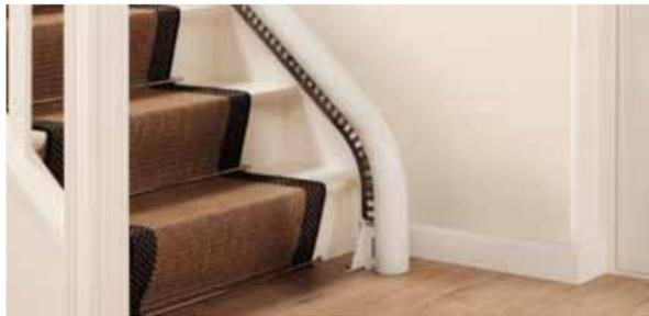
The standard drop nose is the perfect solution if there is an obstruction such as a door near to the bottom of the stairs. The drop nose requires just 175mm of space from the bottom step.
